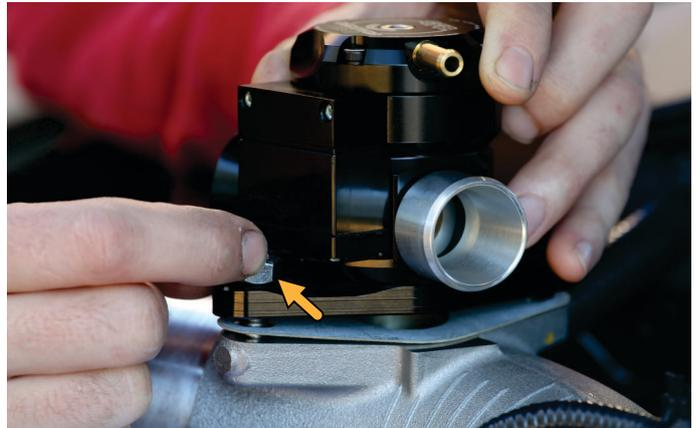
5) Now thread one of the factory bolts into the other hole, then tighten both fasteners fully.
