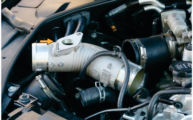
3) Screw the short end of one of the supplied threaded studs into the lower hole of the valve mounting flange as shown opposite ( → ).
