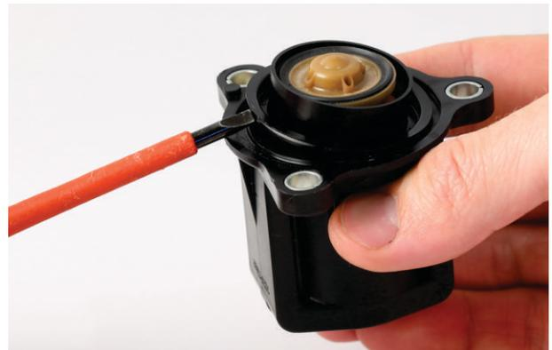
Assemble the GFB parts onto the factory solenoid body as shown in the exploded view below, making sure to use the GFB-supplied plunger spring, and the yellow o-ring removed from the factory valve. Apply some engine oil to the piston during this process, and check that the piston moves freely.
