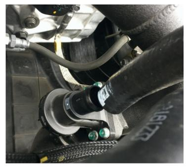
3) Ensure the brown o-ring is installed in the groove on the underside of the Hybrid valve, then install it back in the factory location using the supplied longer screws and 5mm hex key.
