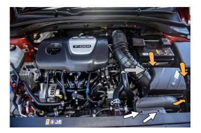
2) Before unbolting the factory valve, it is easiest to first remove the recirc hose while the valve is still solidly mounted (this hose is quite tight and needs some wiggling persuasion). Then remove the factory valve from the car using a 10mm socket for the 4 screws.
