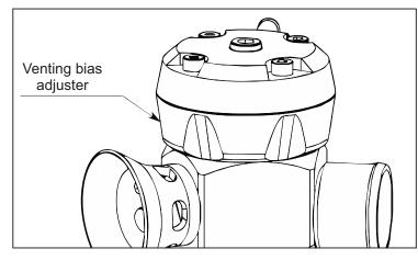
adjustment anywhere in between for a variable venting ratio and to control the sound volume.
