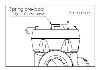
Take the car for a drive, and take note of how easily the valve vents when you lift off. Making the spring softer will allow the valve to open easier and vent longer, and increasing the pre-load means you will need to drive the car harder (i.e. more boost) before you start to hear the valve venting, and the blow-off sound will be shorter in duration.
