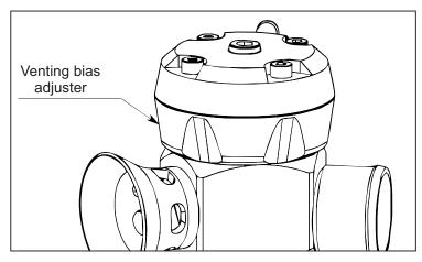
the stock valves and is the quietest operation. You can set the adjustment anywhere in between for a variable venting ratio and to control the sound volume.
