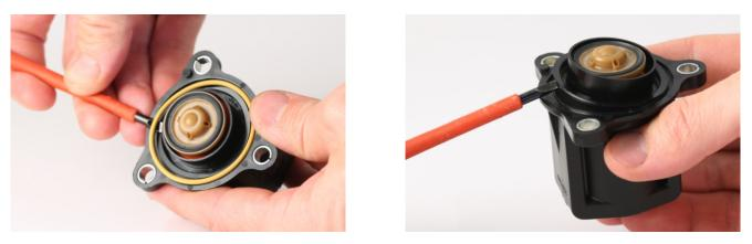
Assemble the GFB parts onto the factory solenoid body as shown in the exploded view below, making sure to use the GFB-supplied plunger spring, and the yellow o-ring removed from the factory valve. Apply some engine oil to the piston during this process.
