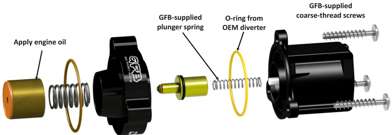
During assembly, check that the piston slides freely in the body without sticking or binding. It is a very close fit and can sometimes be difficult to get started into the bore, but once in it should move without needing to be forced. Apply some engine oil onto the piston during assembly.
