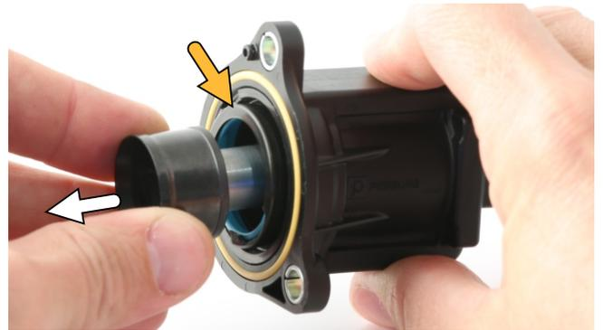
Note that this plastic protrusion is thin and brittle, and damage may occur if levered directly. If it breaks, you'll still be able to continue with the DV+ installation as this part isn't used, but you won't be able to re-install the factory diverter again.
