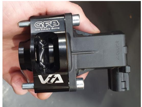
Note that the bolt holes are NOT SYMMETRICAL. When you assemble the VTA onto the solenoid, check the alignment of the holes - if they do not line up properly, rotate the VTA body until the bolt holes line up correctly before continuing.
