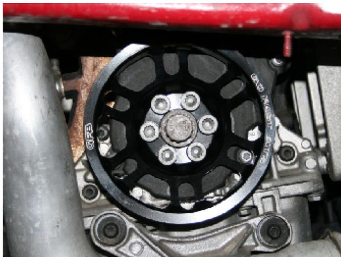
8. For cars with 6mm hex socket bolts – replace the original crank pulley bolts with the ones supplied in the GFB kit along with the washers. For cars with the factory triple square socket bolts, simply re-use them.
