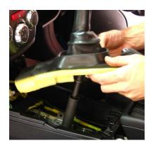
d) Unscrew the plastic buttons that hold the rubber boot/foam insulation, remove it and set aside.
