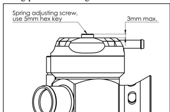
Note that the spring adjusting screw may be obscured by the coil pack when installed, so if adjustments need to be made it is easiest to simply loosen the two valve mounting bolts only enough to rotate the valve up high enough to access the spring adjustment screw, rather than remove the valve entirely.
