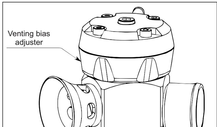
Do not be afraid to experiment with the spring and noise settings, as the Stinger's air/fuel ratio cannot be affected regardless of the BOV settings, and it is not possible to damage the engine or turbos with BOV adjustments.
