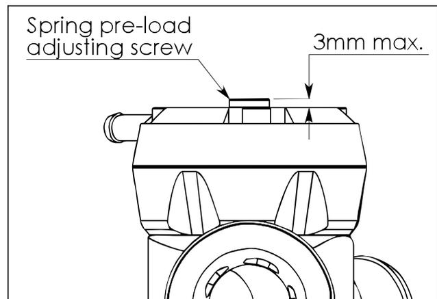
Start by setting the venting bias adjustment to full atmosphere (so you can hear the valves venting during setup - see next page for venting bias adjustment), then set the spring pre-load screws level with the top of the valves.
